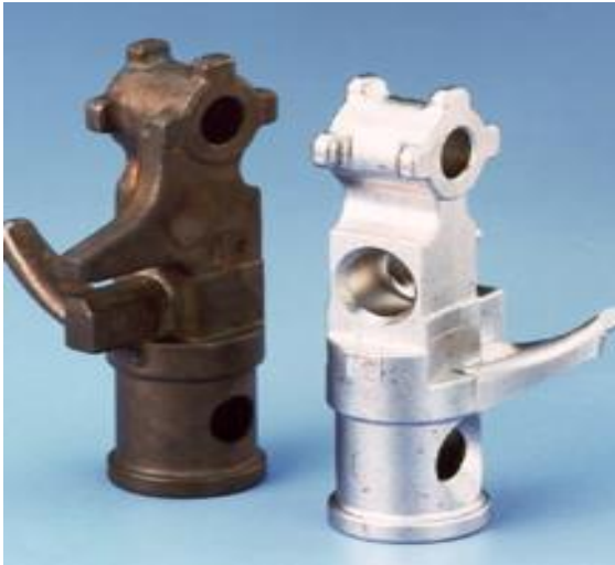
A collection of powder metallurgy parts.
